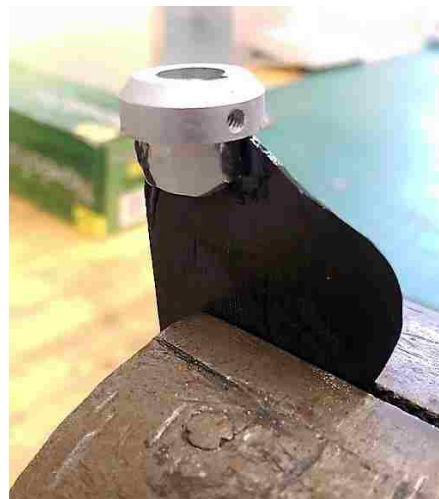
Figure 5.6: Close-up of machined aluminum insert being epoxied to spar
