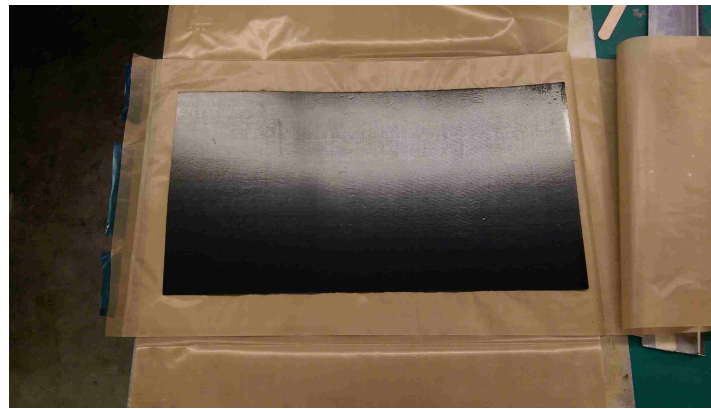
(a) Finished cured laminate from hot press
