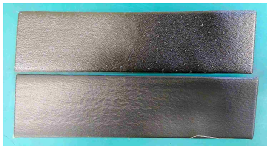
(a) Autoclave-cured laminates used for composite spar
