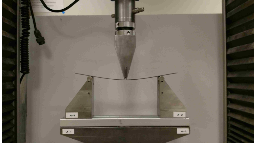
Figure 3.3: 3-point bending experimental setup
